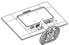
2. Use a flathead screwdriver to remove four mylars from the hinge cover.
