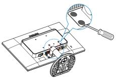
3. Remove the screws from hinge cover.
