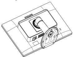
2. Remove the screws from hinge cover.
