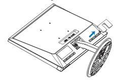
4. Lose four screws to remove the column.
