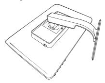
2. Remove the screws from hinge cover.
