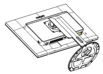
3. While keeping the release button pressed, tilt the base and slide it out.
