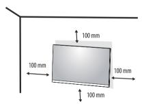
To install the monitor to a wall, attach a wall mounting bracket (optional) to the back of the monitor. Make sure that the wall mounting bracket is securely fixed to the monitor and to the wall.
