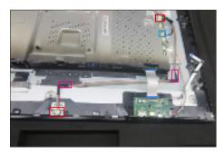
Tear off 1pcs aluminum foil for releasing the USB cable. Use a Philips-head screwdriver to remove 1pcs screw for unlocking the USB unit, then
