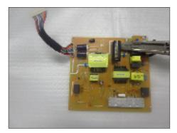
S24-2 Ensure cutting path within the glue, don't touch bulk cap. or PCB.
