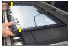
Use a Philips-head screwdriver to remove 4pcs screws for unlocking the left and right Mic boards with the middle frame, then release the two Mic boards away from the middle frame.
