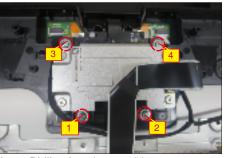
Use a Philips-head screwdriver to remove 4pcs screws for unlocking the bracket chassis with the panel, then disconnect the touch cable.
