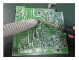
S24-5 Lift the bulk cap. up and away from the PCB.
