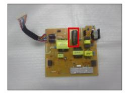
S24-1 Cut the glue between bulk cap. and PCB with a knife.
