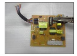
S24-3 Cut into the bottom of bulk cap. and pullit up carefully.
