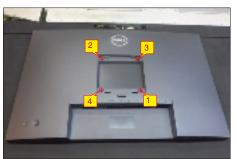
Wedge your fingers between rear cover and the middle bezel on the corners of the top side of the monitor to release the rear cover, then use one hand to press the middle bezel, the other hand to pull up carefully the rear cover in order of arrow preference for unlocking mechanisms of rear cover.
