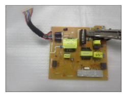
S24-4 Take out bulk cap. pin solder with soldering iron and absorber.
