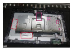
Tear off 3pcs acetate tapes , then disconnect the speakers' cable away from the connector of the main board, and then use a Philips-head screwdriver to remove 6pcs screws for unlocking the two speakers with the middle frame, and remove the speakers. (No.1~6 Screw size= M3x6, Torque=4~5kgfxcm)
