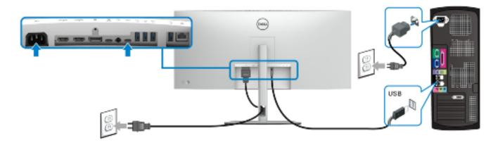
Connecting/ disconnecting the super speed USB 10 Gbps (USB 3.2 Gen2) cable and Power cable
