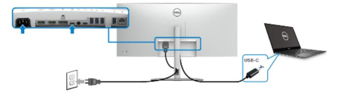
Connecting/ disconnecting the USB Type-C cable (USB-C to USB-A) and Power cable
