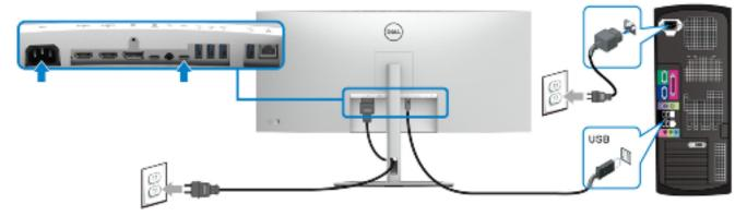
Connecting/ disconnecting the RJ45 Cable (Optional) and Power cable
