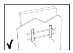
2. After mounting the screen, do not pull, push or shake the screen.
