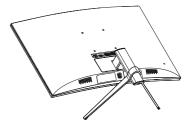
2. Remove the hinge cover from monitor body by using your fingers.
