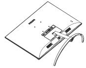
Use your fingers to loosen the screw located at the bottom of the base, and remove the base from the stand
