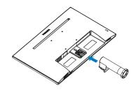
Hold the monitor base stand with both hands and firmly insert the base stand into the base column.
