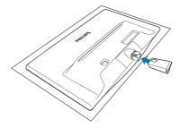
3. Hold the monitor base stand with both hands and firmly insert the base stand into the base column.
