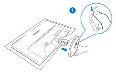
Press the release button to detach the base column.
