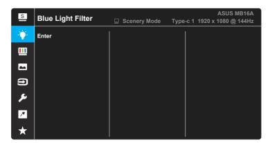
Blue Light Filter: In this function, you can adjust the blue light filter from Min to max. Min: no changes; Max: The higher the level, the less blue light is scattered. When blue light filter is activated, the default settings of Standard Mode will be automatically imported. Besides maximum level, the brightness is user-configurable. Maximum is the optimized setting. It is compliance with TUV low blue light certification\*. The brightness function is not user configurable.
