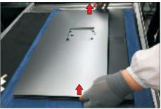
Remove the rear cover and put it on a protective cushion. Use a Philips-head screwdriver to remove 14 screws for unlocking the middle plastic bezel with the whole unit, and then remove the middle plastic bezel carefully.
