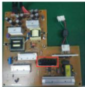
S1 -1 Cut the glue between bulk cap. and PCB with a knife
