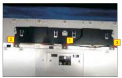
Tear off the aluminum foil for releasing the cooling fans' cable, then disconnect the cable from the connector.
