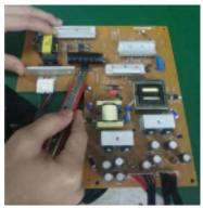
S1 -2 Ensure cutting path within the glue, don't touch bulk cap. or PCB
