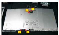
screwdriver to remove 4 screws for unlocking the interface board and LED driver board. Disconnect the cables of the interface board and LED driver board away from the power board, then remove the
