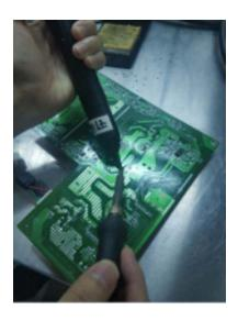
S1 -5 Lift the bulk cap. up and away from the PCB
