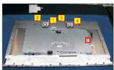
Tear off three pieces of VBH tape on the specific position as the picture below shown. Disconnect the function key cable from the connector of the interface board. Use a Philips-head screwdriver to remove eight screws for unlocking the middle iron bezel with the panel module. Remove the middle iron bezel.
