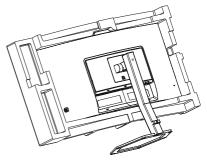
2. While keeping the release button pressed, tilt the base and slide it out.
