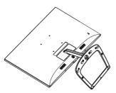
2. Use your fingers to loosen the screw located at the bottom of the base, and remove the base from the stand.
