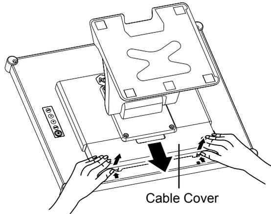
3. After connect the cables to the appropriate connectors and position all cables under the cover lip, attach the cable cover. Take the screw (M3 x 6) from the accessory box, and insert the screw into the cable cover and monitor
