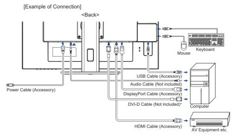
\* DVI dual-link cable is not supplied with the monitor. If you use low quality DVI dual-link cable, it may cause a result of electro-magnetic interference. Please contact the iiyama Support Centre in your country if you wish to connect the monitor via the DVI input.
