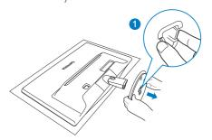
3. Press the release button to detach the base column.
