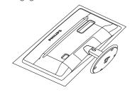
2. Press the locking clips to detach the base stand away from the base column.
