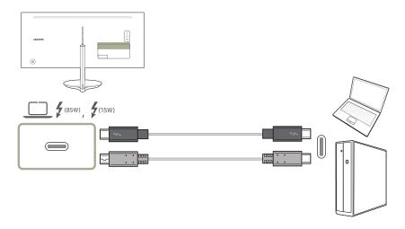
Connect the Thunderbolt  $^{\rm M}$  3 cable or USB Type-C cable to  $\bigcirc$  on the back of the product and  $\bigcirc$  on the PC.
