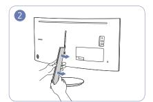
Grab the stand with one hand and use the thumb on your other hand to remove the COVER-STAND NECK LEFT in the direction of the arrow.
