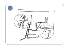
Connect cables to the appropriate ports. Run the cables through the opening on the stand, as shown in the image.
