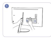
Grab the stand with one hand and use the thumb on your other hand to remove the COVER-REAR-SUB in the direction of the arrow.
