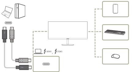
If multiple source devices are connected to the PC, the many cables around the PC may look messy. Connecting the devices directly to the product will resolve such inconvenience.
