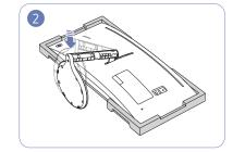
Attach the stand to the back of the monitor, in the direction of the arrow.
