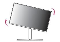
4 Complete the installation by rotating the monitor 90° as shown in the figure.
