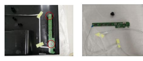
Step.12 Separate wall-mount BKT and display key from rear cover
