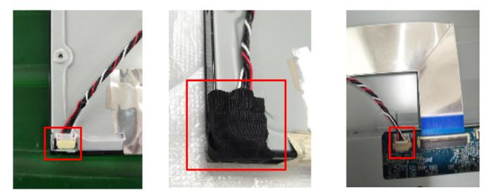
Step6. Insert 10 pin back light FFC and 30 pin LVDS FFC to main board. Use yellow tape to fix.
