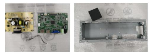
Step.9 Unscrew eleven screws and separate MID FRAME  ${\rm and}\ \text{LCM}$
