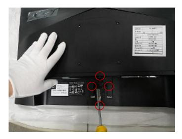
Step.3 Separate hooks between MID\_FRAME and R/C
