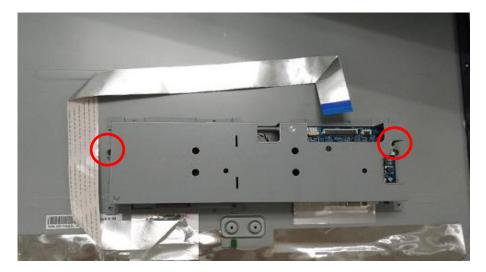
Step4. Use AI tape to fix shielding (tape in blue circle).
