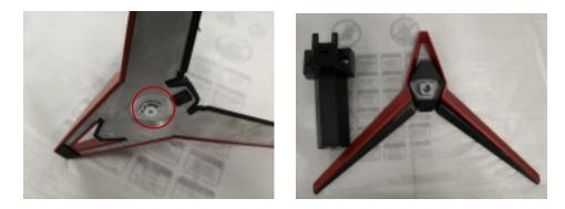
Step.14 Remove four silicon rubbers and unscrew seven screws to separate metal and plastic cover
