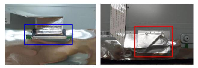
Step3. Lock the shielding on panel with screw. (in red circle)
