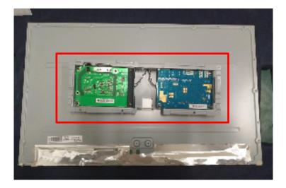
Step2. Insert 30 pin LVDS FFC to LCM, then use acetate cloth tape to tape FFC.
