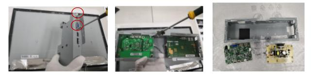
Step.8 Remove connecter cable and separate main board and power board, separate mylar and shielding
