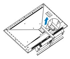
2. Loosen the assembly screws, then detach the stand from the display.
