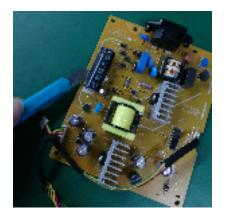
S15-4 Take out bulk cap. pin solder with soldering iron and absorber
