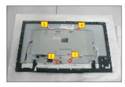
Disconnect the panel power cable to the connector of the panel module. Then disconnect the other cables as the below picture shown.
