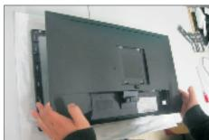
Remove the rear cover. Tear off the aluminum foil, and then disconnect the USB cable and Function key cable away from the connector of the interface board. Use a Philips-head screwdriver to remove one screw for unlocking the USB unit, remove the USB unit from the hooks.
