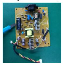
S15-2 Ensure cutting path within the glue, don't touch bulk cap. or PCB
