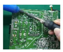
S15-5 Lift the bulk cap. up and away from the PCB
