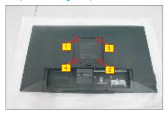
Use one hand to press the rear cover, then wedge your fingers between the rear cover and the middle bezel on the corners of the top left side to the right side of the monitor to release the rear cover.
