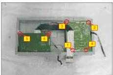
Remove the interface and power boards from the bracket chassis module carefully, and then disconnect all of the cables.
