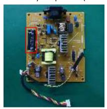
S15-1 Cut the glue between bulk cap. and PCB with a knife
