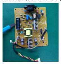
S15-3 Cut into the bottom of bulk cap. and pull it up carefully
