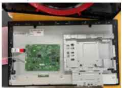
LCD module(together with their casing) is only left after all other parts like electronic units and casing have been removed.
