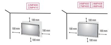
To install the monitor to a wall, attach a wall mounting bracket (optional) to the back of the monitor. Make sure that the wall mounting bracket is securely fixed to the monitor and to the wall.
