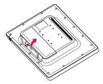
2 After installing the cables, tidy them up using the cable holders.
