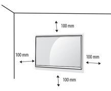
To install the monitor to a wall, attach a wall mount plate (optional) to the back of the monitor.
