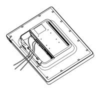
3 Once the back door is attached, assemble it using the screws.
