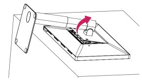
4 Pull the stand away from the monitor in its rotated position.
