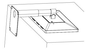
2 Push the Detach button on the back of the monitor to the left.
