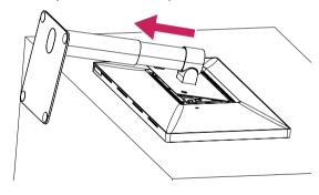
5 Check whether the hooks on the stand are separated from the slots of the main unit.
