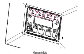
6 Remove the stand once the hooks on the stand have been released from the slots of the main unit.
