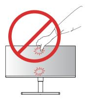
If you use the monitor panel without the stand base, its joystick button may cause the monitor to become unstable and fall, resulting in damage to the monitor or human injury. In addition, this may cause the joystick button to malfunction.
