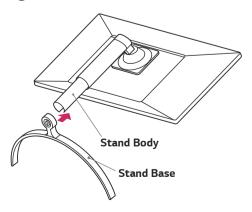
4 Turn the screw clockwise to secure the **stand base**.
