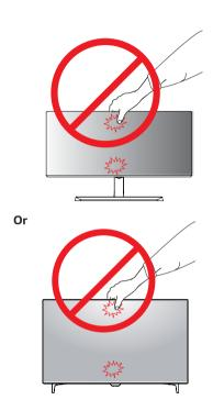
If you use the monitor panel without the stand base, its joystick button may cause the monitor to become unstable and fall, resulting in damage to the monitor or human injury. In addition, this may cause the joystick button to malfunction.
