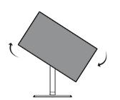
3 Rotate the monitor clockwise as shown in the figure.
