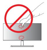
If you use the monitor panel without the stand base, its joystick button may cause the monitor to become unstable and fall, resulting in damage to the monitor or human injury. In addition, this may cause the joystick button to malfunction.
