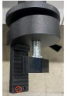
Push button and lift the stand body and remove the screw(4EA)
