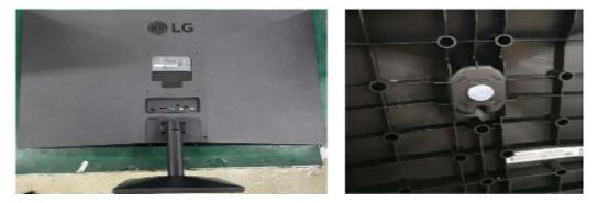
Push button and lift the stand body and remove the screw(4EA)
