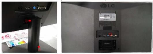
Overturn the set and disassemble the latches of three edges
