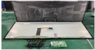
LCD module(together with their casing) is only left after all other parts like electronic units and casing have been removed.
