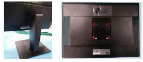
Overturn the set and disassemble the latches of three edges
