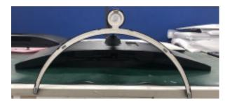
Push button and lift the stand body and remove the screw(1EA)
