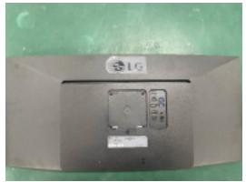
Re-overturn the set and disaaemble screw 4EA and disassemble the PCB
