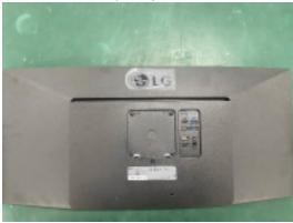
Overturn the set and disassemble the latches of three edges
