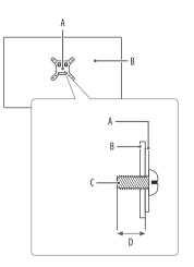
A: Wall Mount Plate B: Back of the Monitor C: Standard screw D: Max. 8 mm
