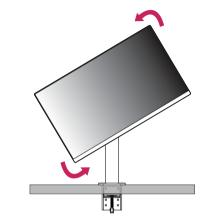
4 Complete the installation by rotating the monitor 90 ° as shown in the figure.
