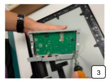
The frame deco can be removed by hand and screw driver.
