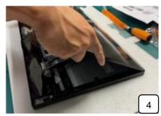
Remove all of connecters, wires and mylar.
