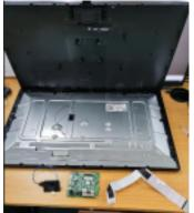
LCD module(together with their casing) is only left after all other parts like electronic units and casing have been removed.
