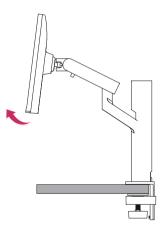
3 Rotate the monitor counter-clockwise as shown in the figure.
