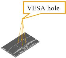
Step 5: Attach the LCD display to the wall, following the instructions in the wallmounting kit. For use only with UL/GS Listed Wall Mount Bracket with minimum weight/load: 8.91 kg
