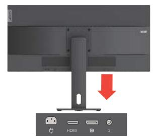
3. Connect one end of the HDMI cable to the monitor HDMI connector and the other end to the computer.
