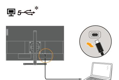
7. Connect one end of the USB cable to the USB downstream terminal of the monitor, and connect the other end of the USB cable to an appropriate USB port on your device.
