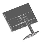
Step 4: Attach the mounting bracket from the VESA compatible wall mounting kit (100mm  $\times$ 100mm distance), VESA Mounting Screw M4  $\times$  10 mm.
