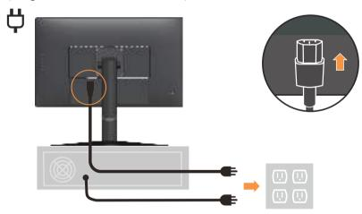
7. Connect the cables with cable clip.
