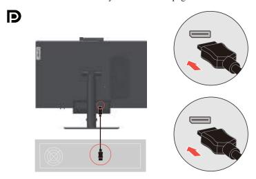
3. Use a type B-to-type A USB cable as shown. Connect type B connector of this cable to the USB 3.0 upstream connector on the monitor. Then, connect type A connector of the cable to a USB connector on the computer. To locate the USB 3.0 upstream connector on the monitor, see "Locating connectors and controls on your monitor" on page 1-5.
