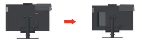
3. Pull the computer out of the computer bay. Then, pivot the cable cover as shown to the closed position.
