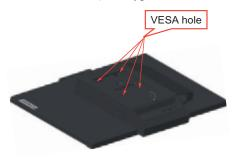
Step 5: Attach the LCD display to the wall, and follow the instructions in the wall-mounting kit.
