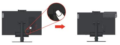
2. Pivot the rear Wi-Fi antenna downward at an angle of about 90°. Then, hold the thicker end of the rear Wi-Fi antenna and unscrew it from the computer.
