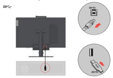
4. Connect one end of the USB cable to the USB downstream terminal on the side of the monitor, and connect the other end of the USB cable to an appropriate USB port on your device.
