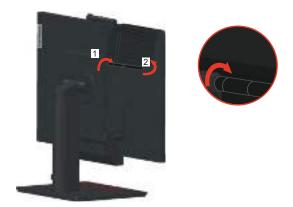
3. Pivot the cable cover as shown to the closed position.
