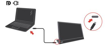
2) Connect the USB-C port of mobile phone and M14t with a USB type-C cable. (Electronically marked cable, current rating: 5A).
