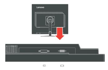
3. Connect one end of the analog signal cable to the monitor D-SUB connector and the other end to the computer.
