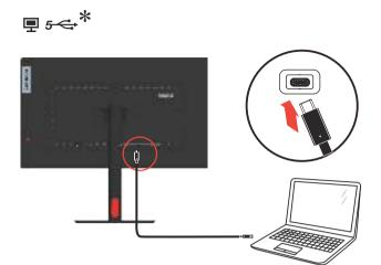
6. For computer in USB type A-C connecting. **Note:** Monitors sold in NA include a USB type A-C cable
