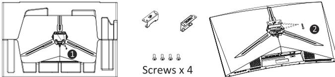
3. Your monitor is now ready to be attached to a wall-mounting bracket. To avoid damage, please do not pinch the screen during bracket installation.
