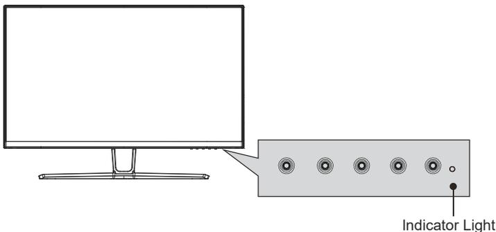
Solid blue light indicates power is on and the monitor is operating normally. Flashing blue light indicates no video source, no horizontal or vertical signal has been detected or voltage is low. Please ensure your computer is on and all video cables are fully inserted and/or connected.
