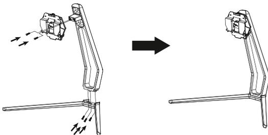
3. As above, vertically push the lock catch. Put stands assembly parts into slot of back cover accordingly and make them mechanically placed. Hold the middle of stand and make sure the monitor won't drop out.
