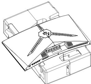
2. Lock the shaft assembly and the bracket with two PM4\*10mm screws, and then lock the three PM4\*10mm screws to the base.
